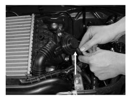
2. Remove the securing bolts and remove the standard BOV
