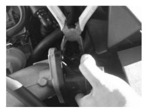
4) Push the plumb back hose onto the plumb back fitting on the new BOV. Use the factory bolts to fit the new BOV onto the intercooler pipe. Remember to install the supplied gasket in between the BOV flange and the intercooler flange. Reinstall the vacuum/pressure source to the nipple.
