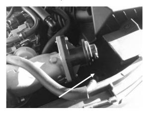
3) Remove the bolts securing the standard BOV and then remove the plumb back hose by removing the spring clamp.
