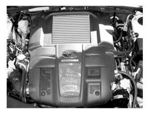
2) Locate standard BOV and remove the plumb back hose and the vacuum/pressure source line.
